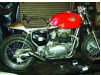
Exhausts look simple but aren’t. Silencing wadding is replaceable without cutting the meggas up
