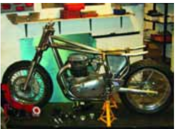
Short motor allowed a 20mm-longer swingarm than the brothers’ other Malarkey-framed machines
