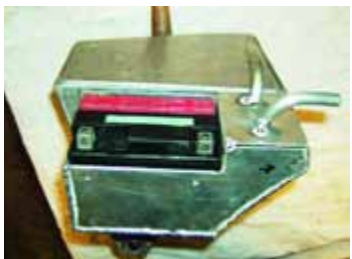
Metal Malarkey’s integral oil tank, breather and battery box. Sorting the breathing was a real headache
